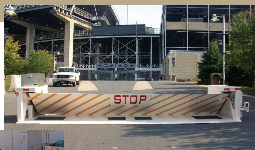
**DSC1000**-A commercial, mobile crash barrier that can be towed into position by a golf cart and deploys in 10 minutes to protect people and property at temporary events ... stops a 5,000 lb (2300 kg) vehicle going 40 mph (64 kph)
